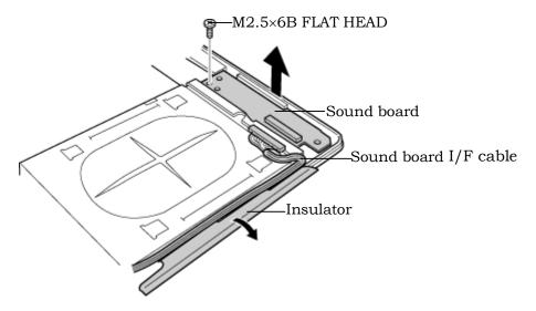
Figure 4-23 Removing the sound board
